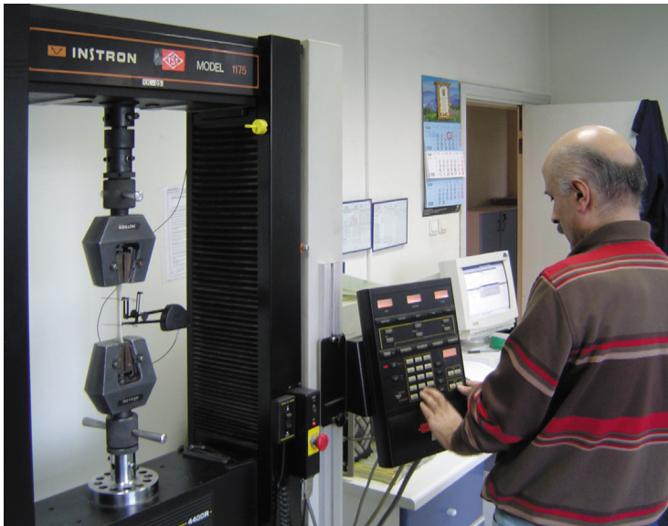
Metyx sample under tensile test
